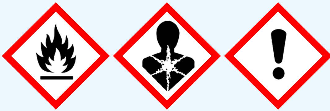
Fig. 7. Pictograms used on labels of ethanol to identify it as a chemical substance, in line with the EU REACH regulation
